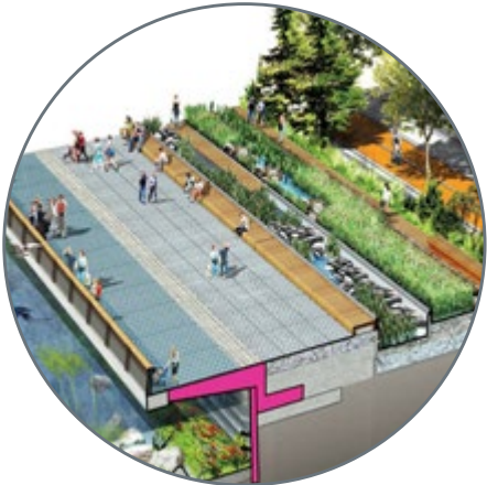
Cross section of new waterfront promenade showing new seawall in pink
